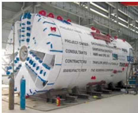
The 4.2 m (13.9 ft) Robbins EPBM will utilize unique PVC inner liner for a sewer project in Sacramento, California, USA
