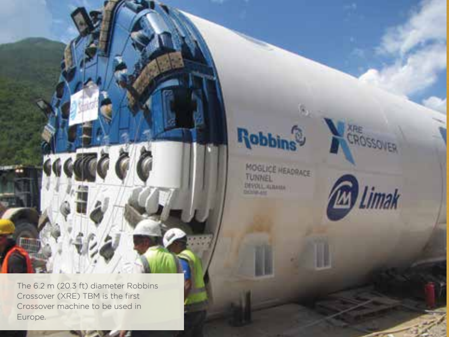
The unique Crossover TBM for the Moglicë Headrace Tunnel is sealable up to 20 bars and is made to excavate through challenging mixed ground conditions.
