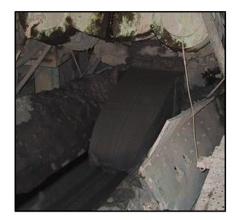
Figure 9. Well-conditioned clay leaving the screw conveyor onto the belt conveyor (photo courtesy of Mapei UTT)
