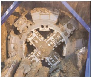
Figure 1. EPB machine with severely clogged cutterhead in adhesive soil.
