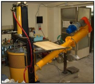
Figure 5. Testing fixture. Treated sample is placed in barrel on left and subjected to pressure and extracted from barrel through screw conveyor on right. (Photo courtesy of Mapei-UTT)
