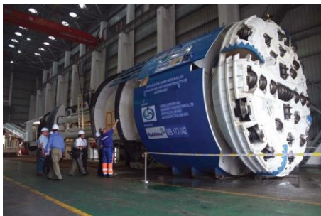
Figure 1. Main Beam or Open-Type TBM for competent rock
