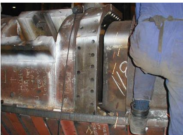
Figure 14. Muck Bucket Gate Closed for Double Shield TBM.
