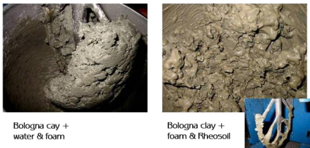
Figure 10. Anti-Clay Additive (courtesy of BASF)
