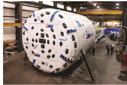
Figure 3. Single Shield TBM for very fractured rock
