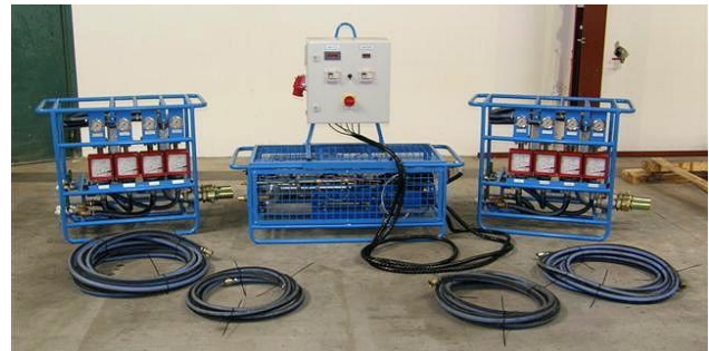
Figure 11. Manual foam system (courtesy of BASF)
