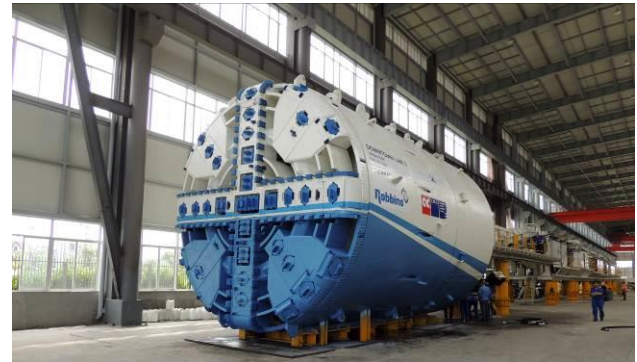
Figures 11. The first of six EPBS assembled in Pudong, China.
