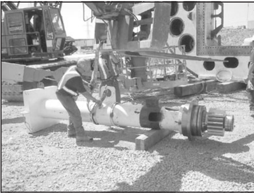
Figure 3. Special tool for installation of final drive pinions
