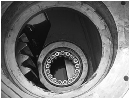
Figure 16. Installation of drive pinions—Mexico MX12
