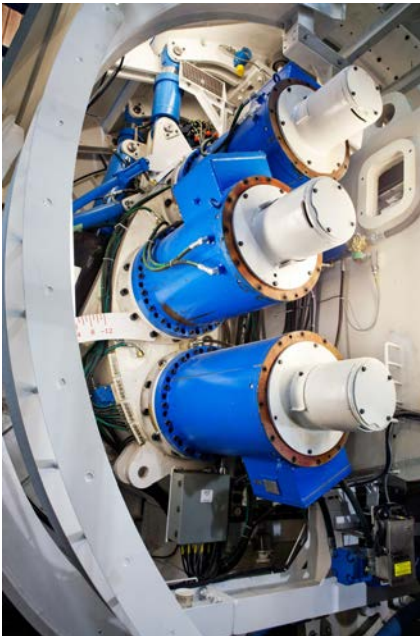
Fig. 6. VFD setup in a hard rock TBM
