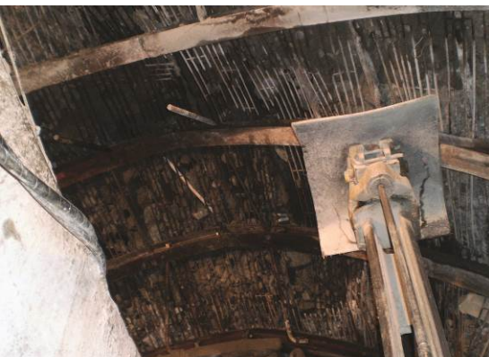
Figure 15. Steel Slats containing Rock Bursting
