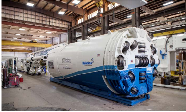
Figure 3. View of Robbins Ø3m Double Shield TBM used on Rosemont Project
