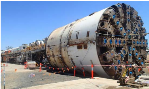
Fig. 20. Transport Drift - TBM ready for re-launch and soft ground tool dress
