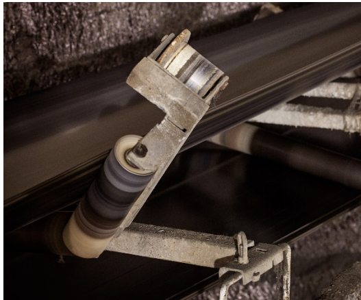
Figure 7. Close-up of self-adjusting curve idler Figure 8. A view of one of the 90-degree curves
