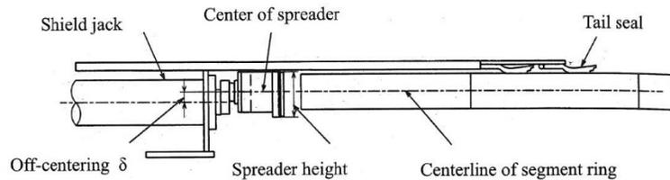
**Figure 4. Shield jack with off-centering rod end**
