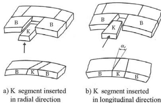
**Figure 3. Insertion angle of the K-segment**
