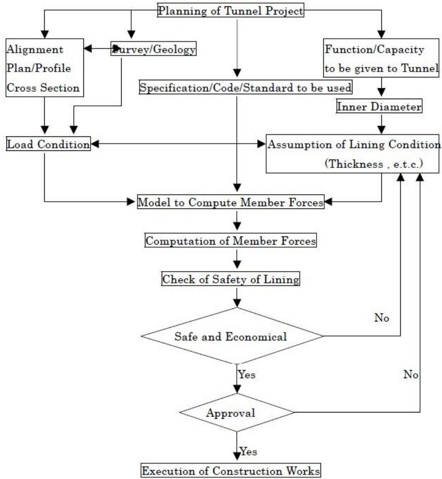
Figure1. Segment design workflow
