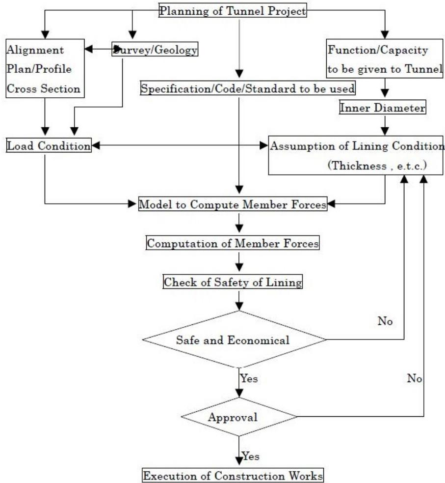
Figure1. Segment design workflow
