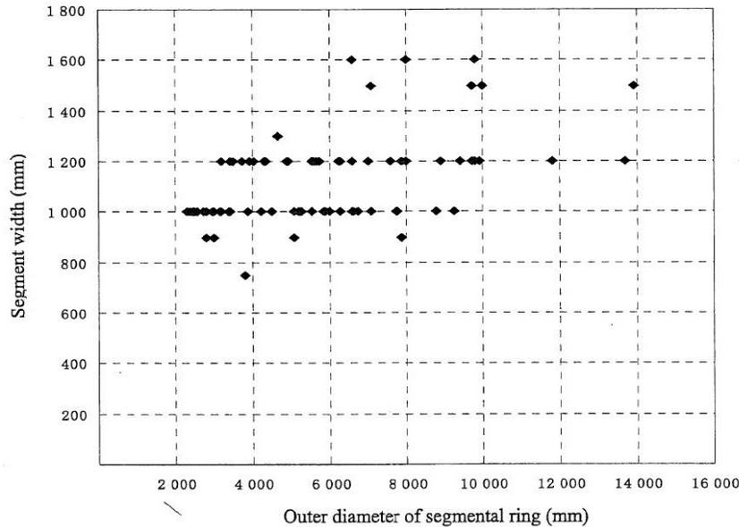
**Figure 2. Trend of segment width compared to segment outer diameter**
