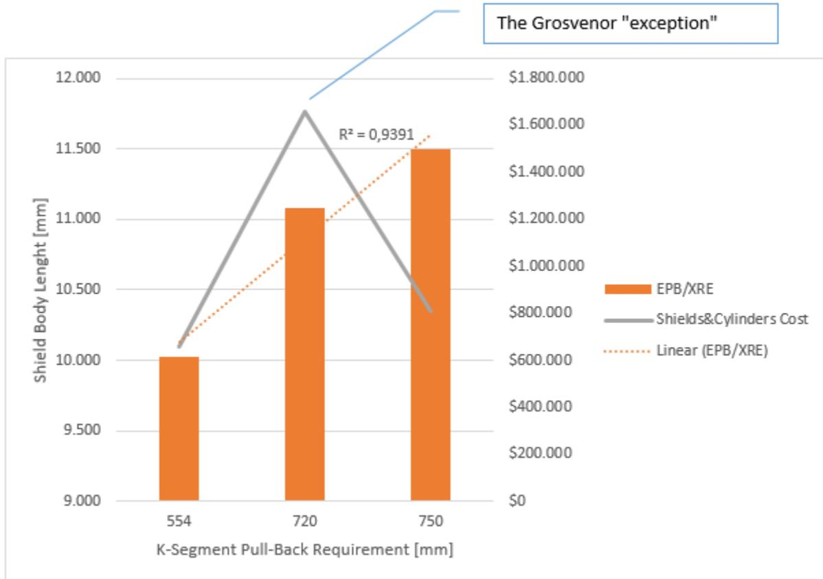
**Figure 10. EPB segment width compared to shield body length and cost**
