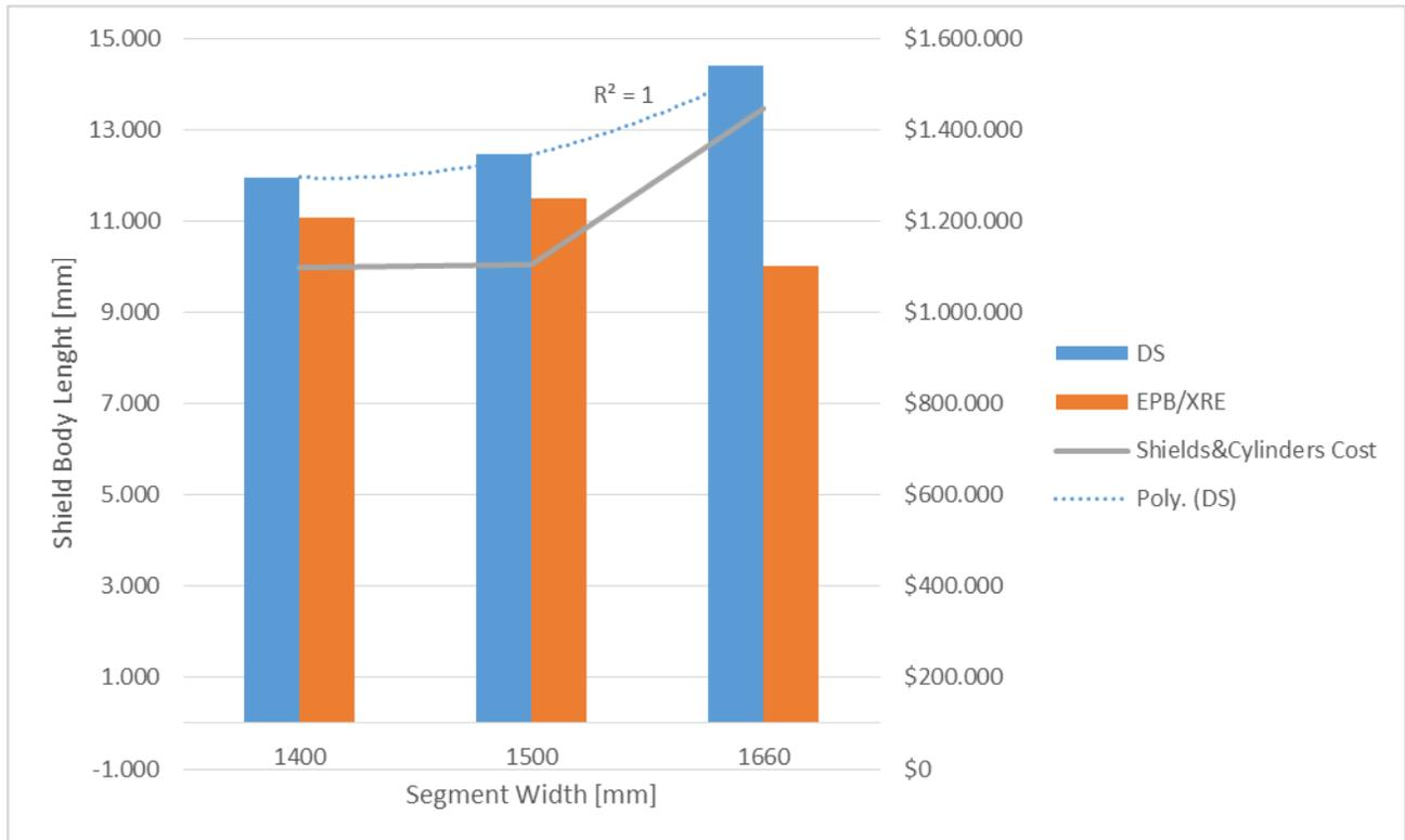
**Figure 9. DS segment width compared to shield body length and cost**
