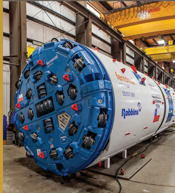
Mid-sized Double Shield TBM in the Solon, Ohio, USA manufacturing facility
