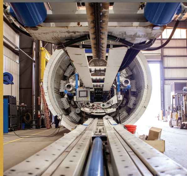
Rear view of a Double Shield TBM showing segment erector
