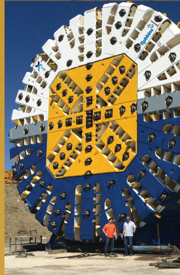
Large diameter XRE TBM with cutterhead set up for rock conditions
