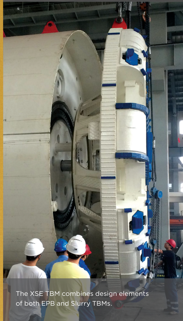
An XSE TBM with customized cutterhead designed for mixed ground conditions.
