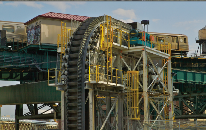
An efficient S-type vertical conveyor operates at New York City's East Side Access Project
