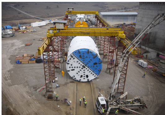
Figure 1. 10 m diameter Double Shield TBM for the Kargi HEP
