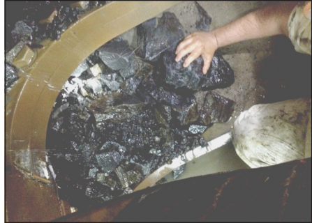
Figure 19. Blocky material (andesite with fine sand from weathered rhyolite) inside the cutterhead
