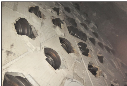
Figure 3. Cutterhead installed with US-manufactured 20-inch cutters
