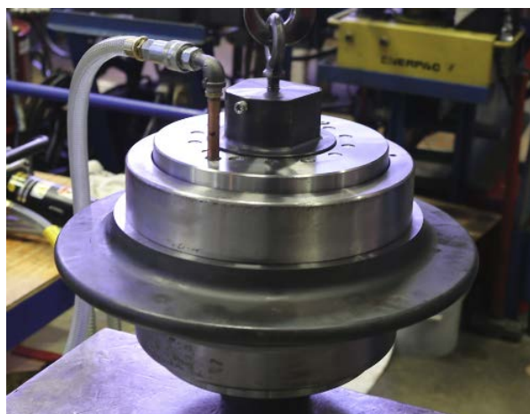
Figure 6. Pressure compensating disc cutter.
