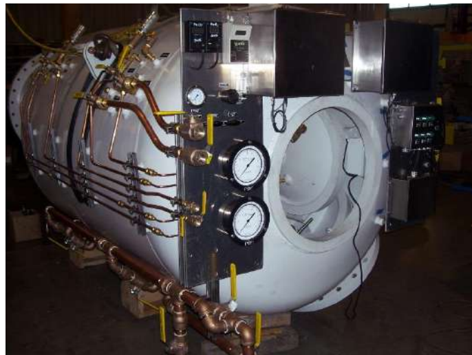
Figure 9. Man Lock for 7 bar pressure.
