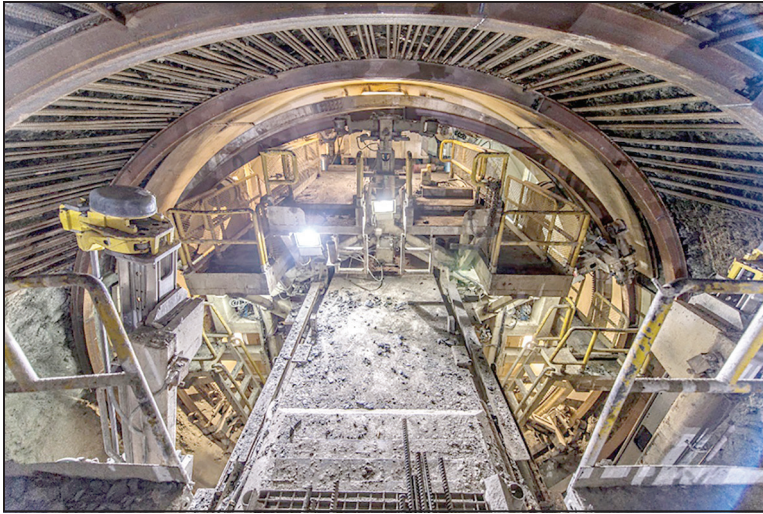
Figure 2. The McNally roof support system utilizes steel slats extruded from pockets in a TBM's roof shield
