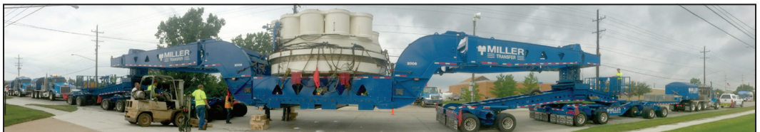
Figure 8. Cutterhead support on the 15-axle dual lane truck
