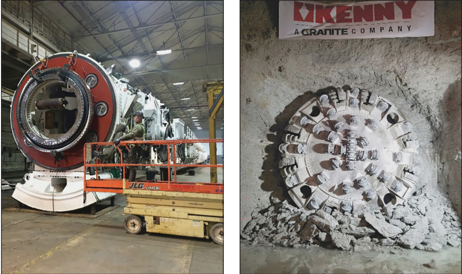
Figure 1. A main beam TBM originally built in 1979 was refurbished and successfully completed the Albany Park Stormwater Diversion Tunnel in Chicago, IL, in late 2017
