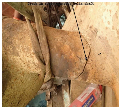
Figure 7. Extreme wear of helix measured at 230 mm to inside of casing & cracks at screw helix shaft.
