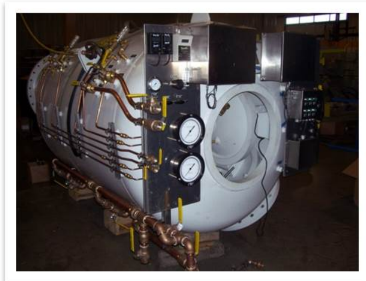
Figure 9. Man Lock for 7 bar pressure.
