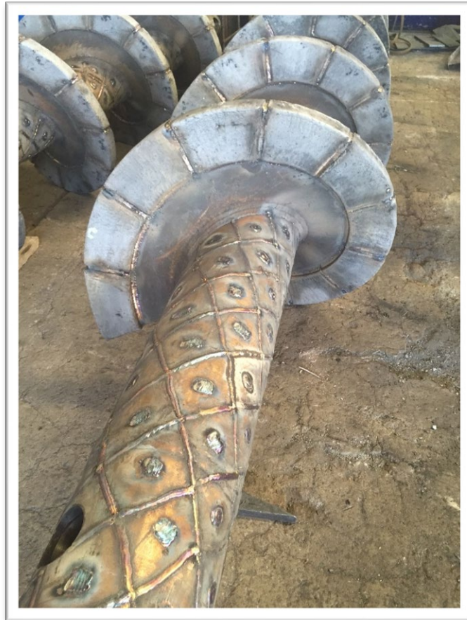
Figure 12. Screw Conveyor Helix Wear Protection plates.
