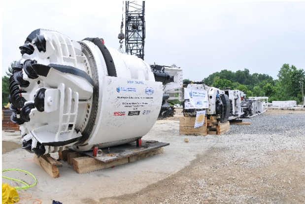
Figure 5. “Miss Colleen”, the Main Beam TBM for the Bi-County Water Tunnel
