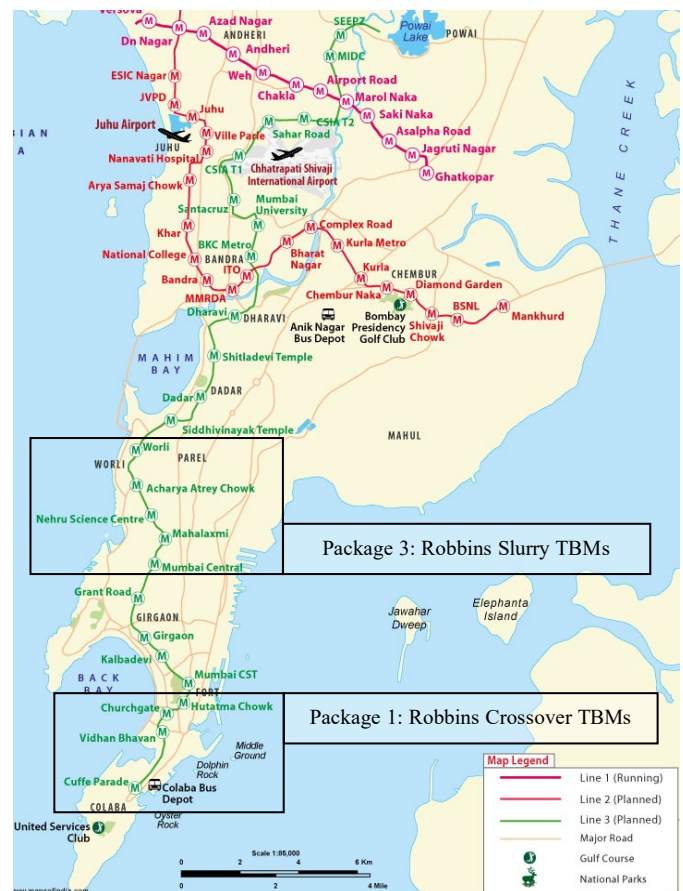
Figure 1: Robbins TBMs at the Mumbai Metro line 3 project
