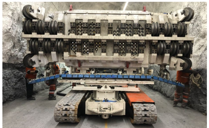
Figure 7. MDM cutterhead on a mobile, tracked carrier
