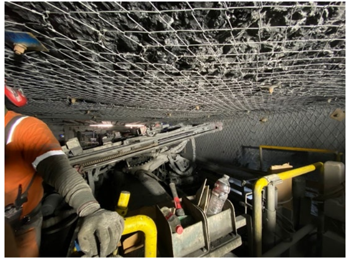
Figure 9. Hydraulic percussive drills for roof bolting
