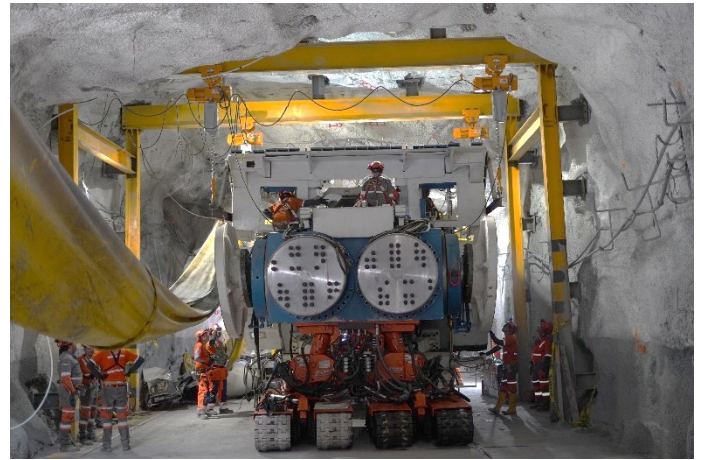
Figure 11. Main frame of MDM on transport crawlers inside assembly chamber area
