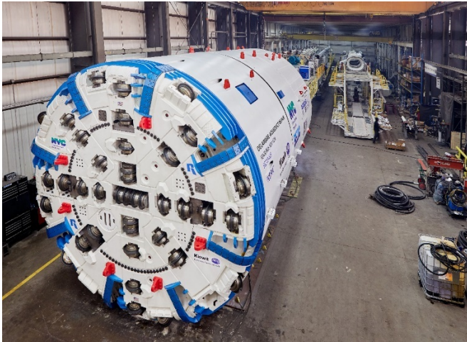
Figure 2. The 6.58 m (21.6 ft) diameter Delaware Aqueduct Repair TBM, a Single Shield machine used in hard rock and designed to statically hold high water pressure, is a good example of NCP tunnelling.
