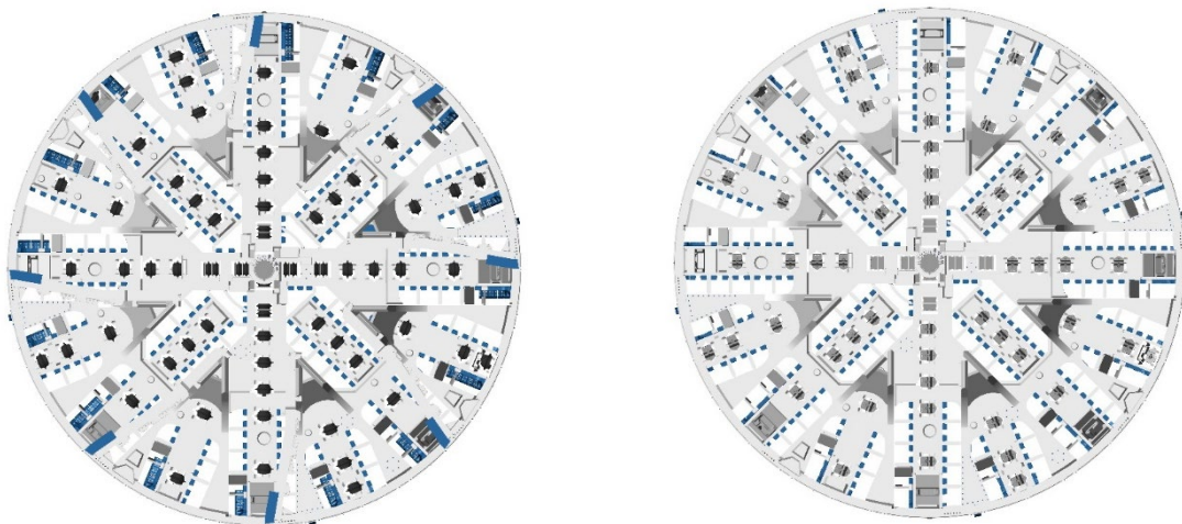
Figure 3. Left Cutterhead in Rock Configuration; Right Cutterhead in EPB Configuration
