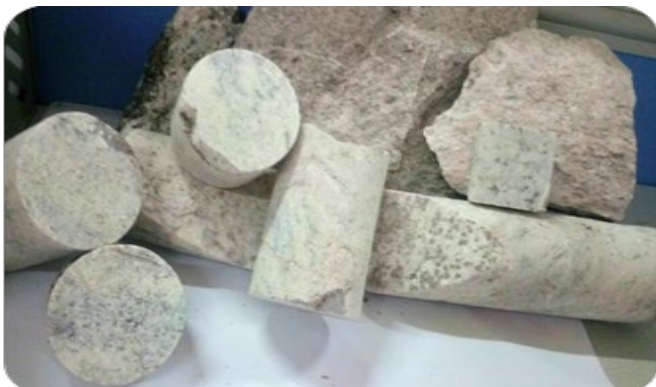
Figure 5. Quartz granitoid core samples analyzed.
