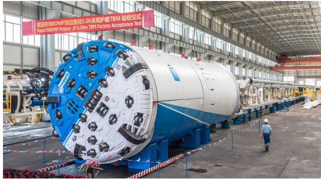
Fig. 4. BBDMP TBM in factory in Shanghai, China
